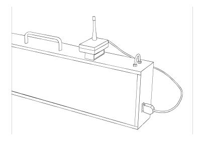
To attach the wireless interface unit to the top of the scoreboard, simply press straight down onto the Velcro – you will feel the unit click into place.
