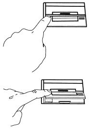
2. Push down on the right side of the ribbon cartridge marked "PUSH". Remove the cartridge.
