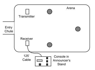
The Transmitter unit is labeled "Transmitter" on its rear panel. The Transmitter outputs the infrared light beam that is detected by the Receiver. The infrared light is emitted through the solid black front panel. The Transmitter has built in rechargeable batteries to allow operation in the arena without AC power. However, if by mistake the batteries were not charged, the Transmitter can be operated by plugging it in.
